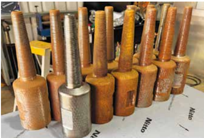
Slika 2: Odstranjena površinska rja (Perth Laser Cleaning, 2025). Untitled design – rust removal sample [Photograph]. PerthLaserCleaning Website. https://perthlasercleaning.com.au/wp-content/uploads/2024/12/Untitled-design-2024-12-05T112938.855-800x534.png
